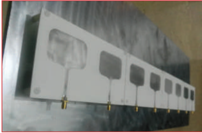
▲ Fig. 4 Eight-element monopole array.
