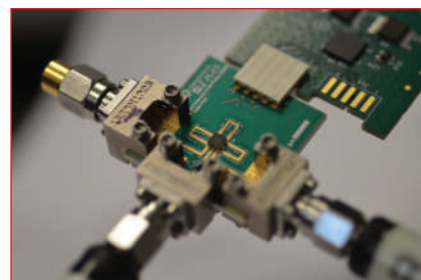
▲ Fig. 8 Testing the differential delay shifter prototype.
